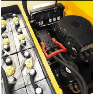
Drive and lift motor with 3-phase AC technology
