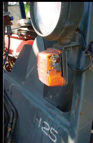
X – Unacceptable lens damage
