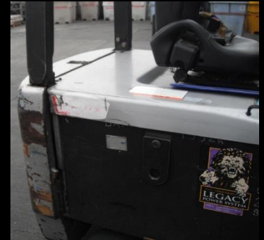
X – Unacceptable dents to A battery cover
