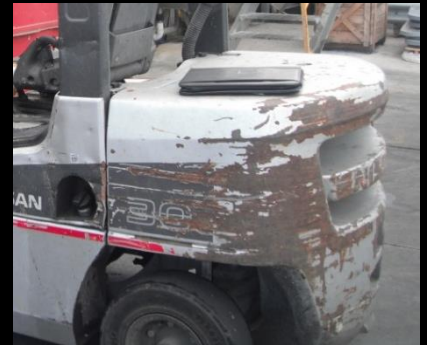
X – Unacceptable paint damage
