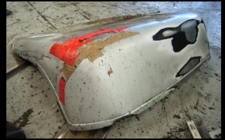
X – Unacceptable damage to a bonnet
