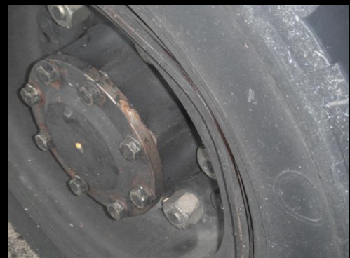
X – Unacceptable lock ring damage
