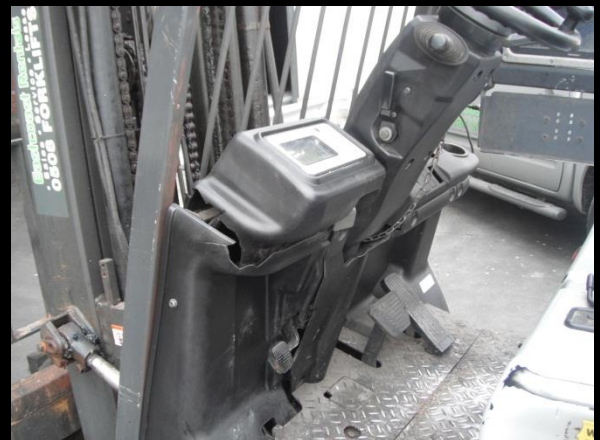
X – Unacceptable customer damage. Cracked and broken guard, missing
