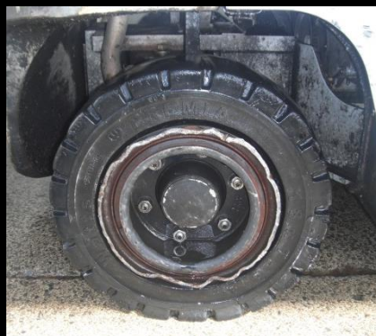
X – Unacceptable lock ring damage
