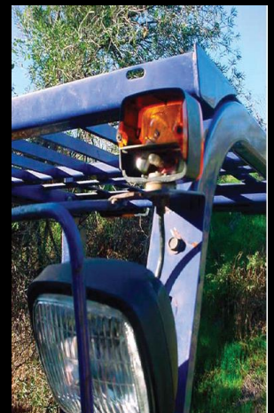
X – Unacceptable lens damage
