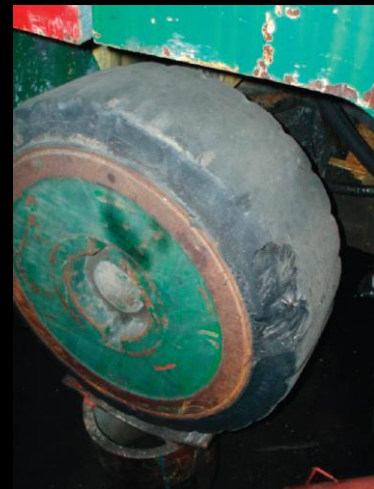
X – Unacceptable Tyre cut
