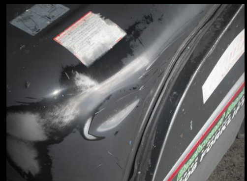
√ – Acceptable wear and tear. This paint has worn off from the driver entering and exiting the machine. The paint rubbing near the seat caused by legs and hands when considering the age and hours of the machine is acceptable wear and tear
