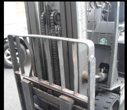
X – Unacceptable damage to a load guard
