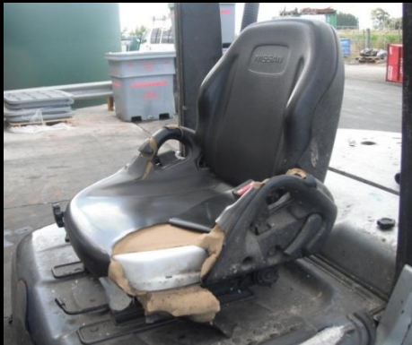
X – Unacceptable damage to a seat
