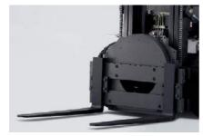
**Rotating Fork** Full 360° rotation, for faster work and easier load
