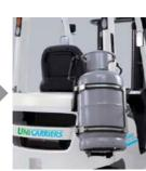
This ergonomically designed swing-down bracket greatly assists in for the lifting and lowering of tanks. The improved design also provides better rearward visibility (available on all LPG-powered models).
