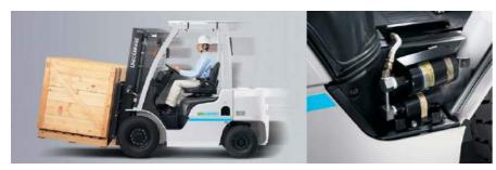
Two different types of accumulators absorb the shocks transmitted from the road surface making both load handling and travel smoother. This offers extra benefits when working with delicate loads on rough surfaces.
