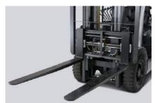
A hook-type fork positioner, for accurate positioning of the forks with the load.
